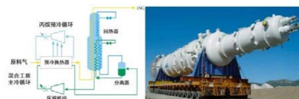
图4 C3MRC 天然气液化流程和大型缠绕管式液化冷箱 图源：Air Products & Chemicals, Inc., Linde Plc.
